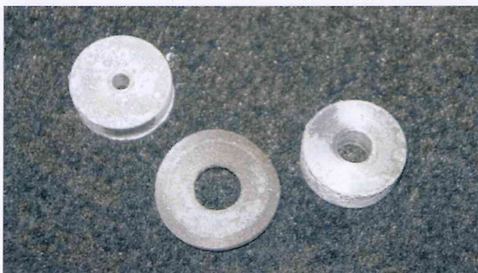
Pictures of the EUT and electrodes oxidation after 96 hours SST
