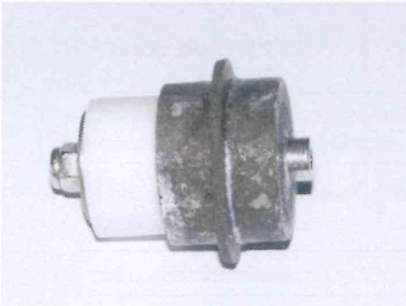
Oxidation of aluminum electrodes after 48 hours SST.
