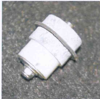
Pictures of the EUT and electrodes oxidation after 96 hours SST
