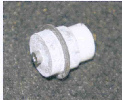
Pictures of the EUT and electrodes oxidation after 96 hours SST
